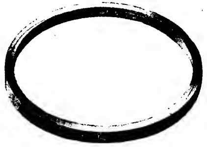
Hi-Comp piston ring composed of two eccentric interlocking rings
